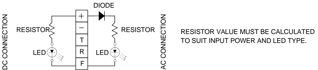
FIG. 3: FLASH OUT CONNECTIONS TO EXTERNAL LED
